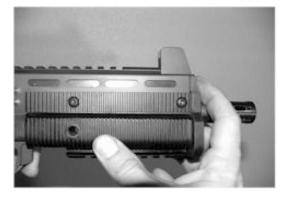
7 Push retaining pin through right side until fully seated.
