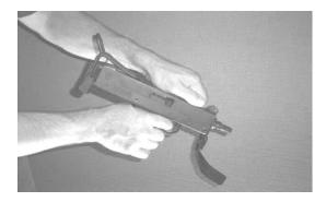
3 Remove front pushpin and detach upper receiver from lower receiver.
