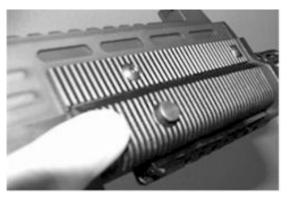
(3) Hold upper and lower receiver together with one hand and with other hand grasp protruding head of retaining pin and pull out.
