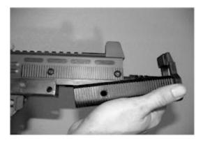
(6) Slide grip back and insure front of grip locks in under front sight and hole in grip sides align with receiver hole.
