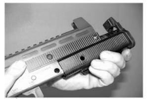
(5) Remove upper receiver from lower receiver.
